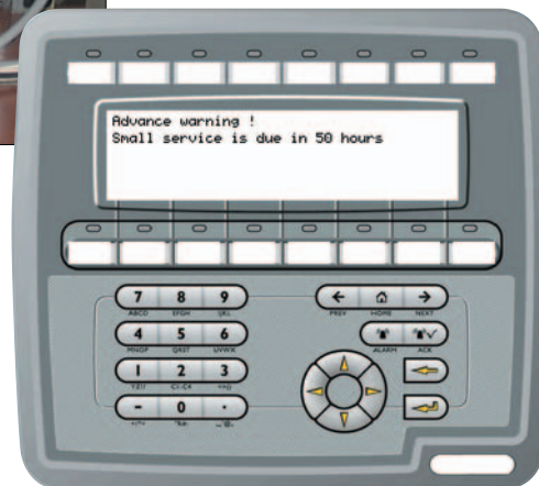
The maintenance and inspection module monitors the machine and will betimes remind of necessary inspections. Maintenance work can be organised without disturbance of the production.
