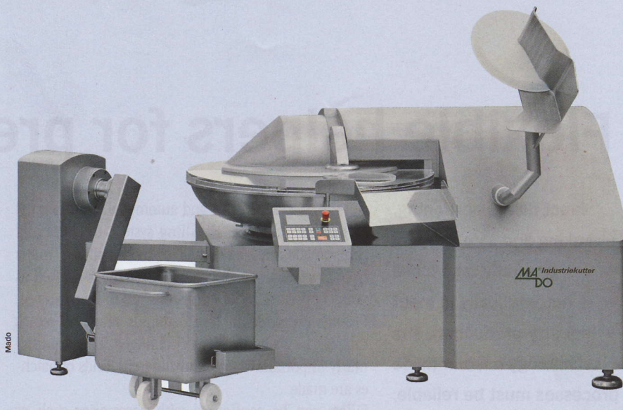
The Supra MSM 769 SL cutter-mixer has an infinitely variable knife shaft with speeds ranging from 50 to 5,000 rpm.
